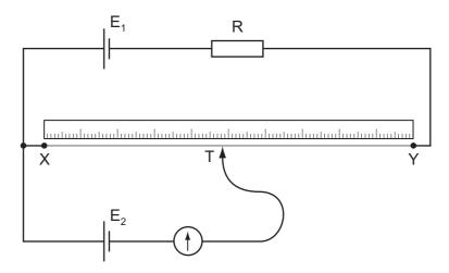
The contact T is placed on the wire and moved along the wire until the galvanometer reading is zero. The length XT is then noted.
